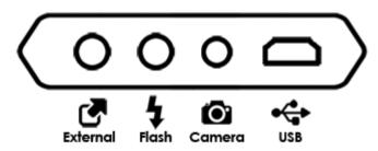
The camera cable port is a 2.5 mm stereo female jack. The camera cables have the male 2.5 mm stereo jack on one end. This end is plugged into the camera connection port. The other end changes depending on the camera make and model. This end is plugged in the shutter release port of your camera.
